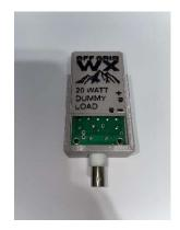
3. Attach the back cover. If you want to make the assembly permanent, then put one small dab of glue or epoxy in the middle of each of the four sides of the back cover that insert into the case. Otherwise, the friction fit seems sufficient to prevent the cover from coming off.
