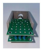
on the bottom of the case that matches up with the flat section of the BNC adapter on the circuit boards.
